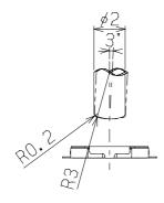
Operating area: Within 1mm from the center of the switch Allowable incline of operating: Less than 3 degree
