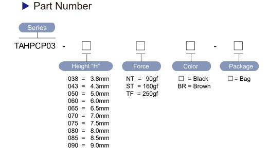
TAHPCP03Series4.5\*4.5mm Tact Switch, Through, Side actuator
