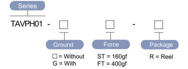
TAVPH01Series3.0\*2.7mmTact Switch, Reflow, Top actuator
