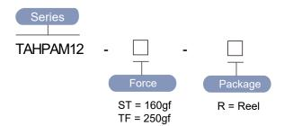
TAHPAM12Series4.5\*2.5mm Tact Switch, Reflow, Side actuator
